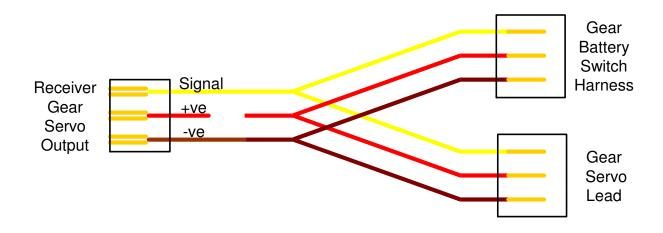
Note that +ve wire is cut near to the Receiver connection so that current will flow from the Gear Battery directly to the Gear Servo. This method ensures that the two batteries are not connected in parallel but share a common –ve connection with the receiver. Remove a section of the wire as pictured to prevent accidental shorting.
